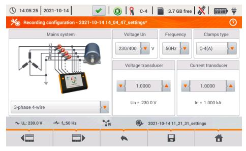
Fig. 6. Recording configuration – General settings
