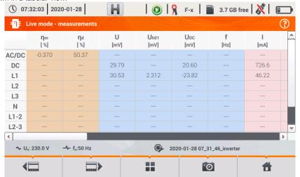
Fig. 47. Live mode in tabular view for the inverter efficiency measurement mode.
