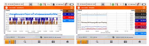
Fig. 48. Screens for waveforms and timeplots in the mode of inverter efficiency measurement
