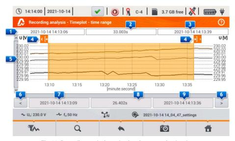
Fig. 23. Recording analysis - selecting time range for the chart.
