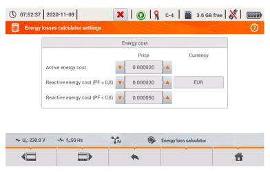
Fig. 51. Energy loss analysis - configuration screen 2
