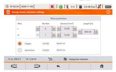
Fig. 50. Energy loss analysis - configuration screen 1
