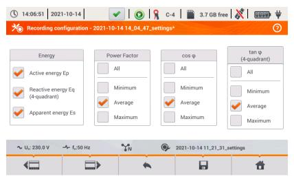
Fig. 11. Recording configuration – Energy and power factors
