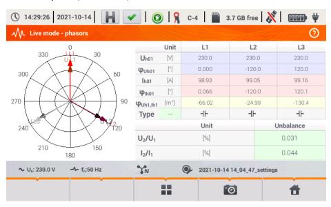
Fig. 55. Live mode - phasor diagram.
