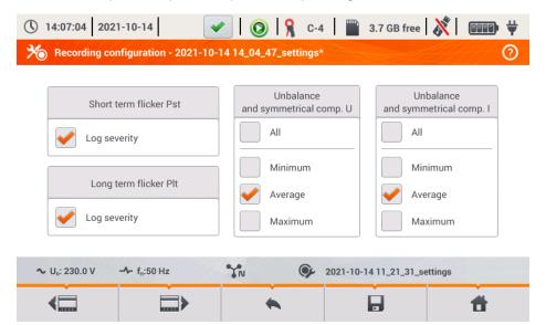
Fig. 12. Recording configuration - Flicker factor and asymmetry.
